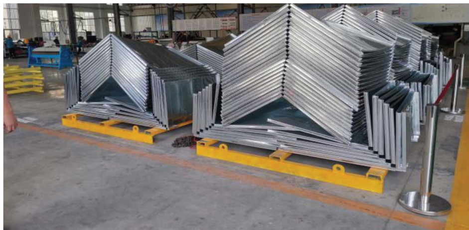
Figure 4. Semi-finished air duct
