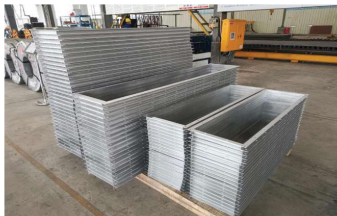
Figure 3. Finished angle steel flange
