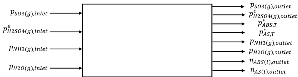
Figure 2. Variables at the inlet and outlet of the reactor under high concentration feed
