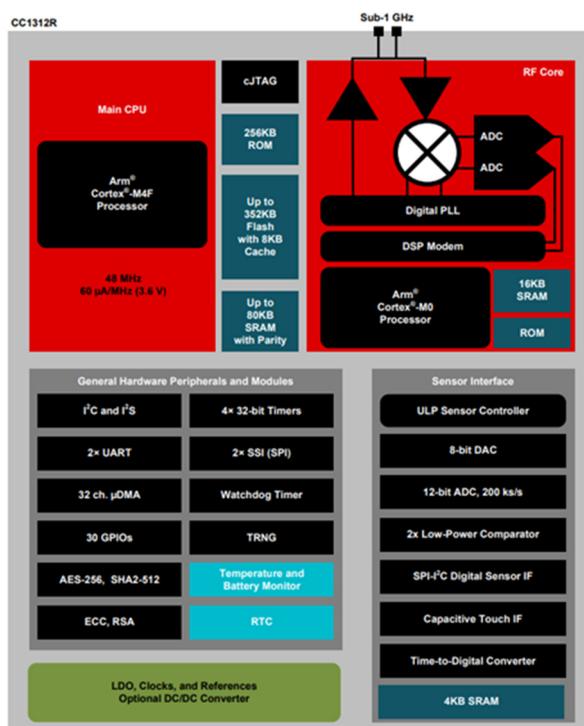
Figure 1. CC1312R module diagram
