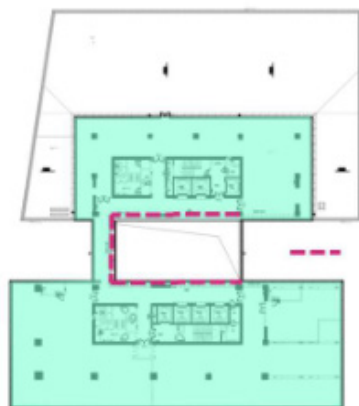
Figure 5. Three-layer fire protection zone
