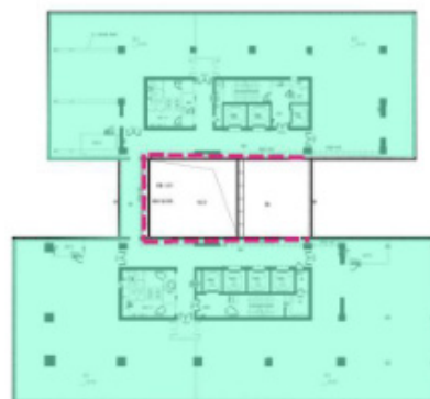
Figure 6. four-layer and above fire protection zone
