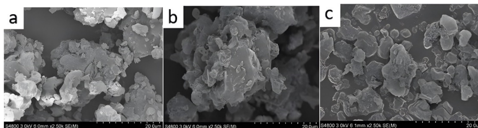
Fig 1. SEM images of (a) \text{Ti}_3\text{AlC}_2 , (b) \text{Ti}_3\text{C}_2\text{T}_x , and (c) \text{MoS}_2\text{-Ti}_3\text{C}_2\text{T}_x
