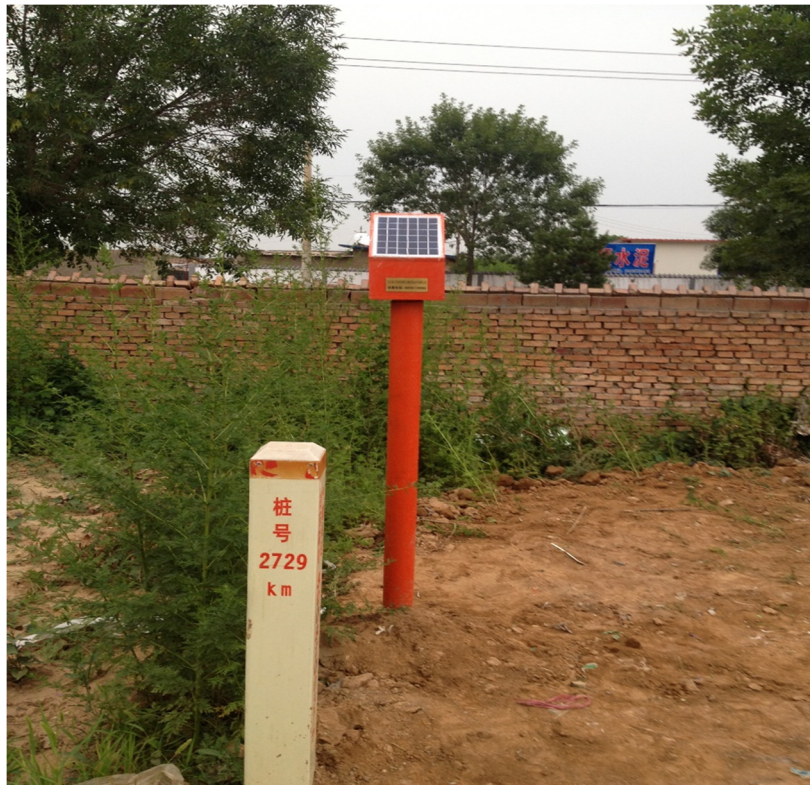
(b) Field detection pile for pipeline geological hazards
