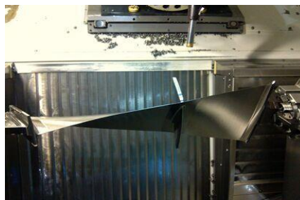
Figure 1. Precision milling of blades
