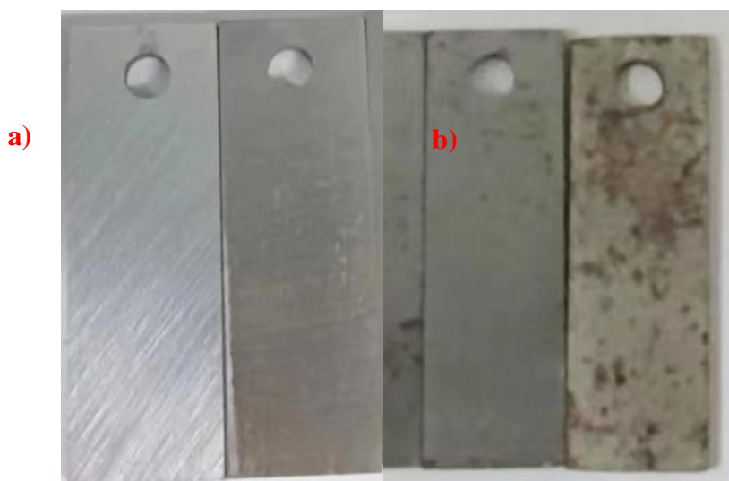
Fig. 3 Different forms of Q235 steel sheet before and after the hanging piece experiment
