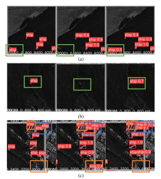
**Fig.** 5 Comparative experiments of BiCBAM-YOLOv5 and the traditional YOLOv5 for ship detection in nearshore (a) and ocean (b) and port (c).
