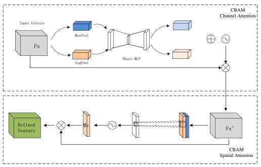
Fig. 3 The structure of the attention modules
