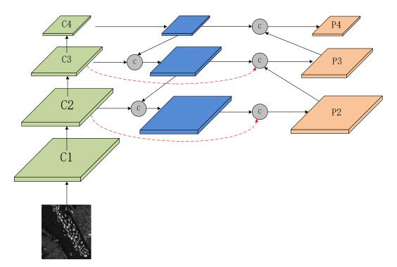
Fig. 2 The framework of the pyramid based approach
