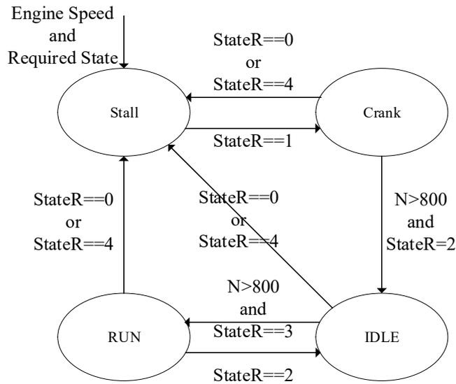
Figure 6. Working condition switching
