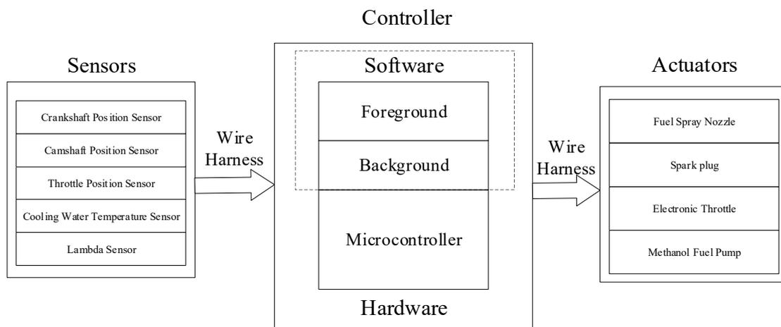
**Figure 2.** The overall structure of the control system
