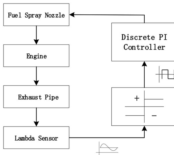
Figure 7. The principle of air-fuel ratio closed-loop control
