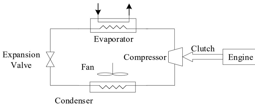
Figure 1. Working principle of heat pump system
