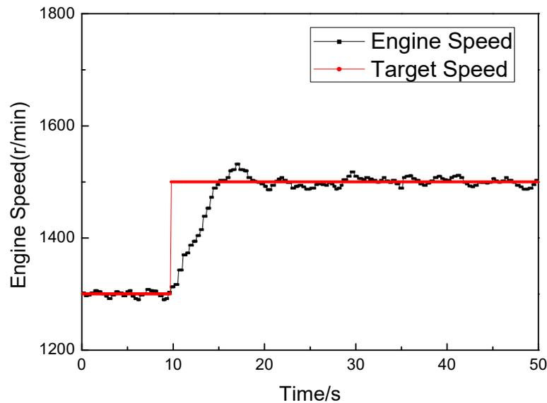
Figure 10. Results of speed adjustment test
