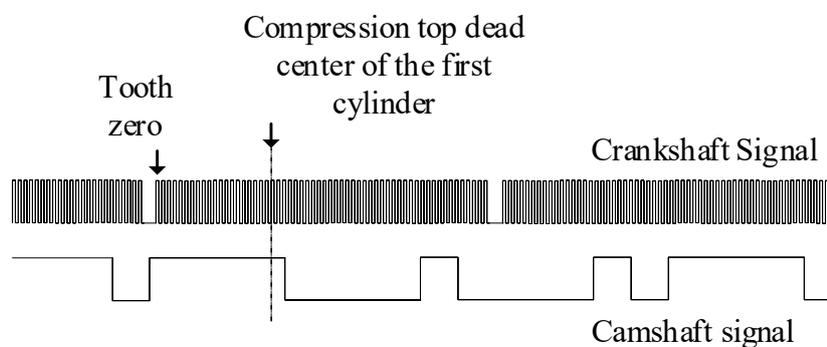
**Figure 3.** The relative position relationship between the crankshaft signal and the camshaft signal
