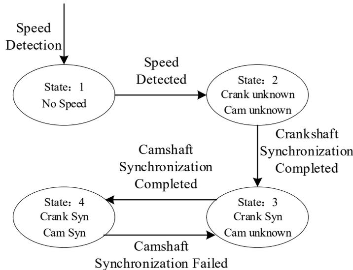
Figure 4. Synchronization algorithm state switching
