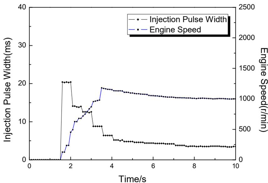
**Figure 9.** Results of engine start test
