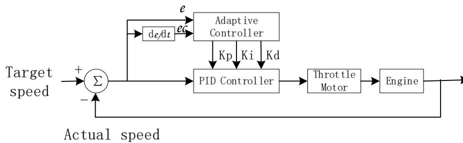
**Figure 8.** Algorithm of adaptive PID control
