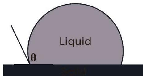
Fig. 1. Illustration of contact angle.
