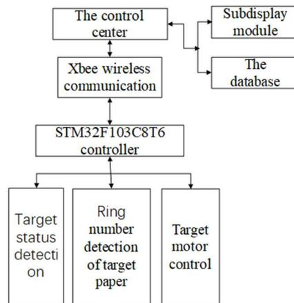
Figure 1. System logical architecture
