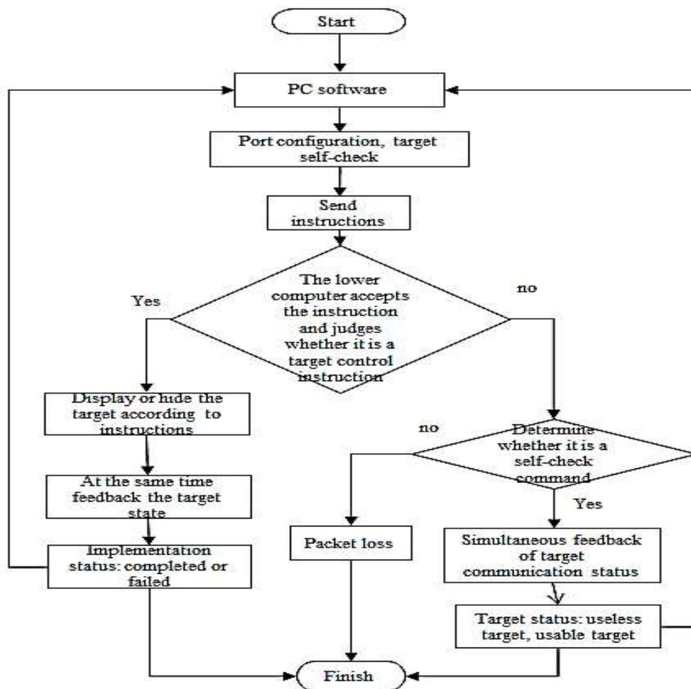
Figure 5. System software control design process
