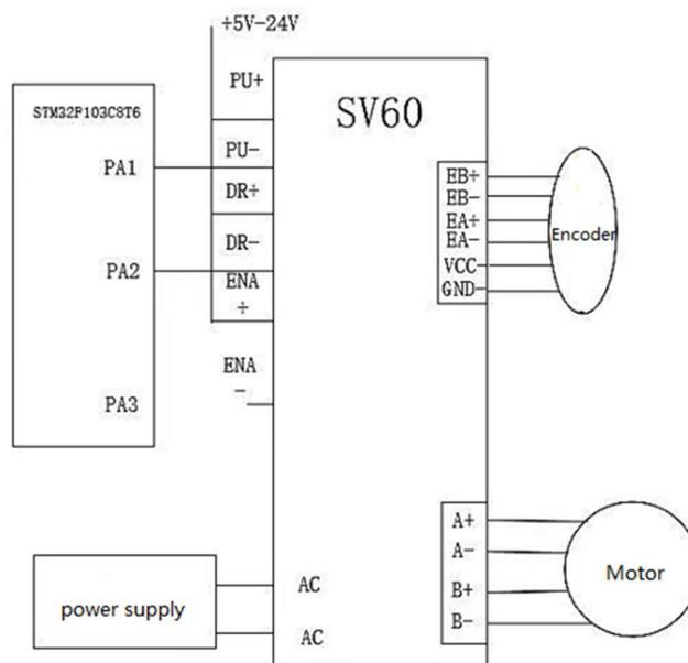
Figure 2. Motor drive control wiring diagram
