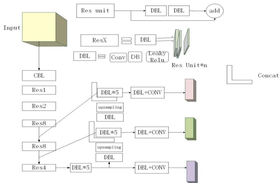
Fig. 4. The structure of yolov3
