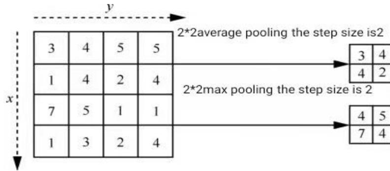
Fig. 2. Schematic diagram of pooling process
