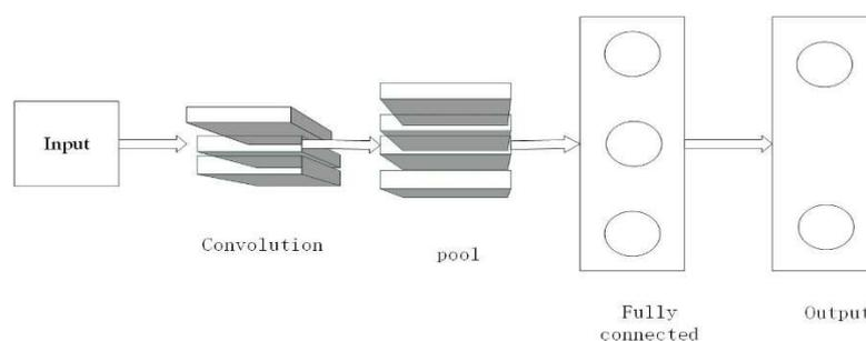
Fig. 1. The structure of CNN
