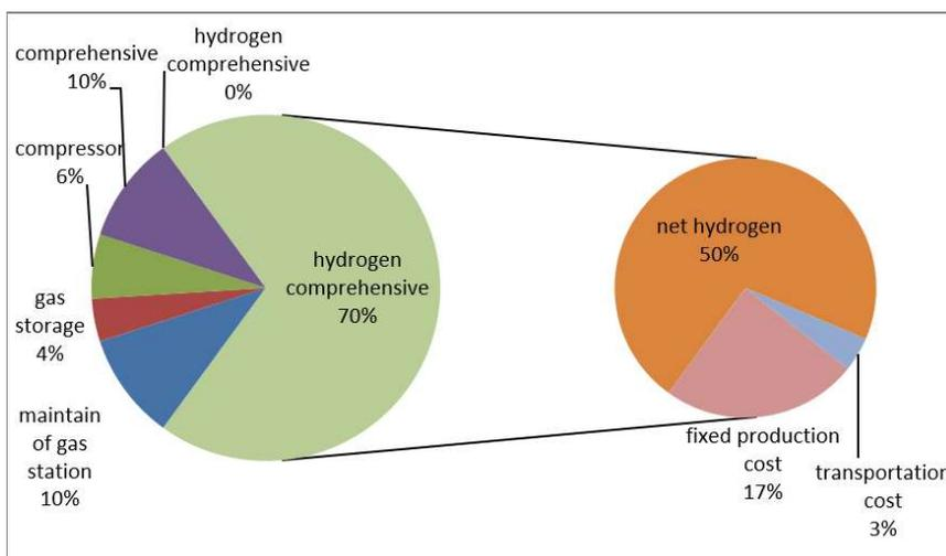
**Figure 1.** Hydrogen cost accounts for 70% of the selling price of hydrogen
