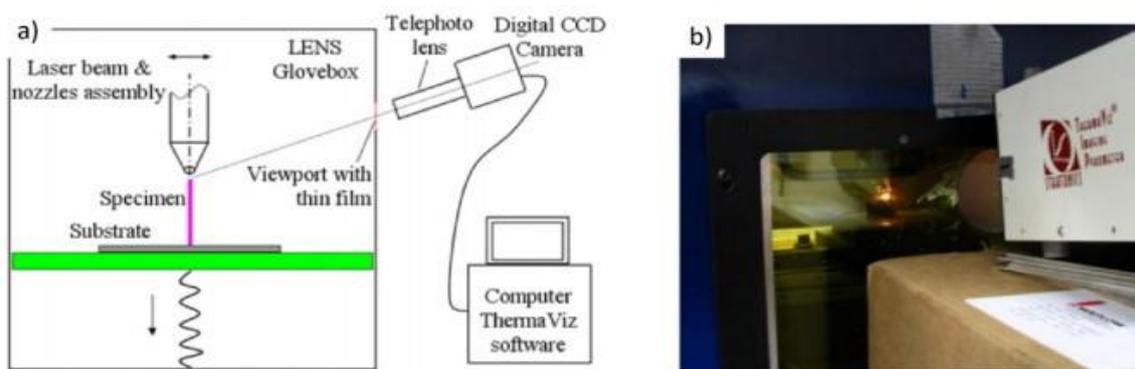
Figure 2. (a) schematic of digital CCD camera focussed through viewpoint for thermal behaviour analysis and (b) photograph of set-up selected by Wang et al. [10]
