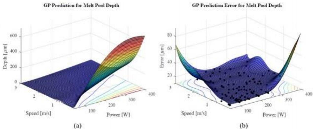
Figure 3. (a) The process map of melt pool depth in terms of laser power and scan speed of 316 stainless steel in L-PBF process, and (b) the corresponding uncertainty
