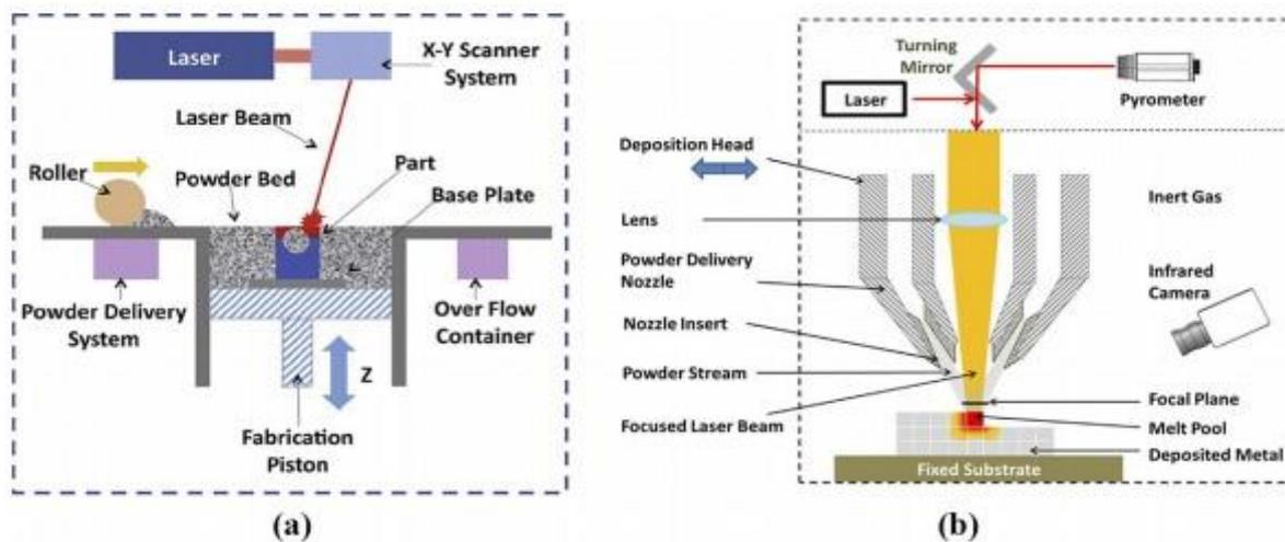
Figure 1. (a) Schematic diagram of powder bed fusion (PBF) and (b) schematic diagram of directed energy deposition (DED)
