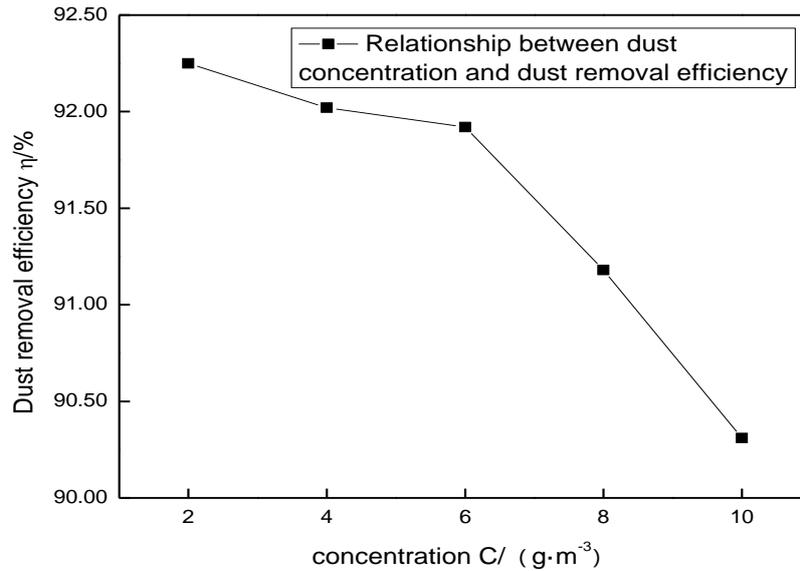
Fig. 8 Concentration and total dust removal efficiency
