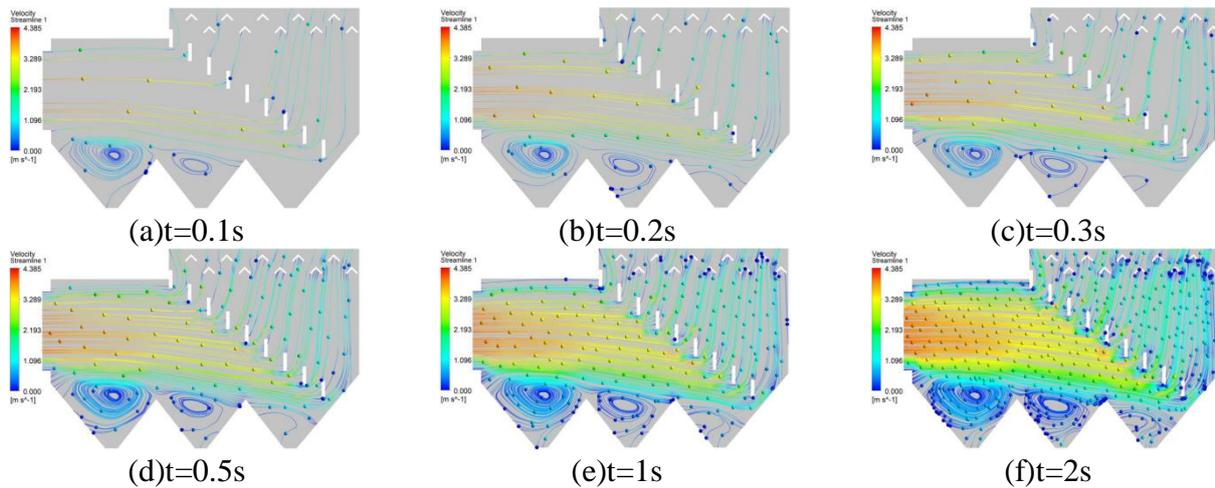
Fig. 4 Particle streamline trajectory diagram of the central section of the computational domain
