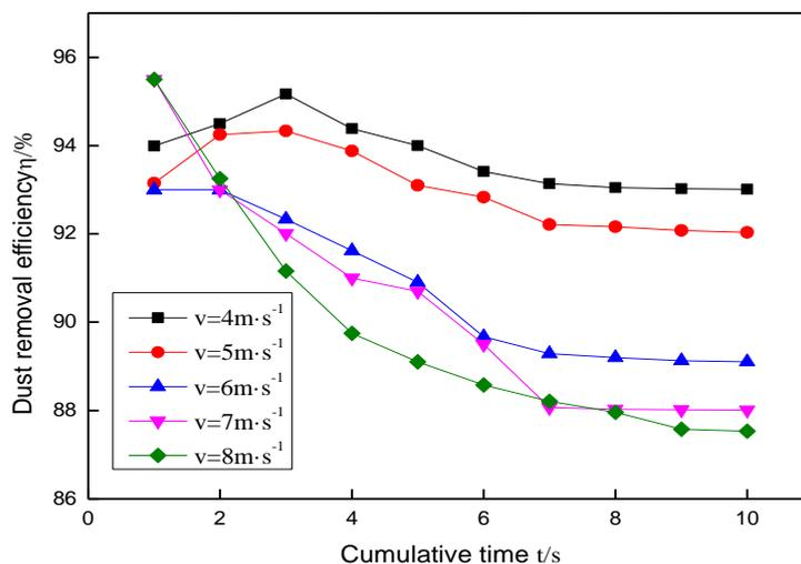
Fig. 5 The influence of different speeds on dust removal efficiency
