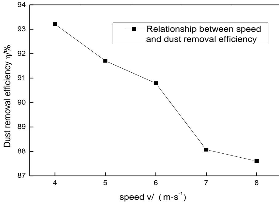
Fig. 6 Speed and total dust removal efficiency
