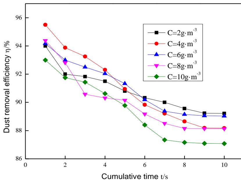
Fig. 7 Influence of different concentrations on dust removal efficiency
