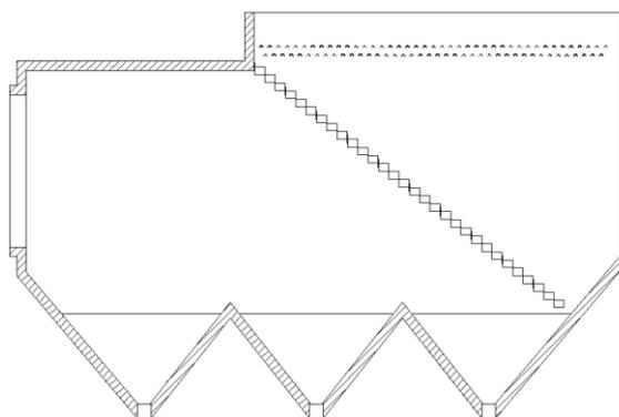
Fig. 1 Schematic diagram of cement kiln waste heat boiler structure
