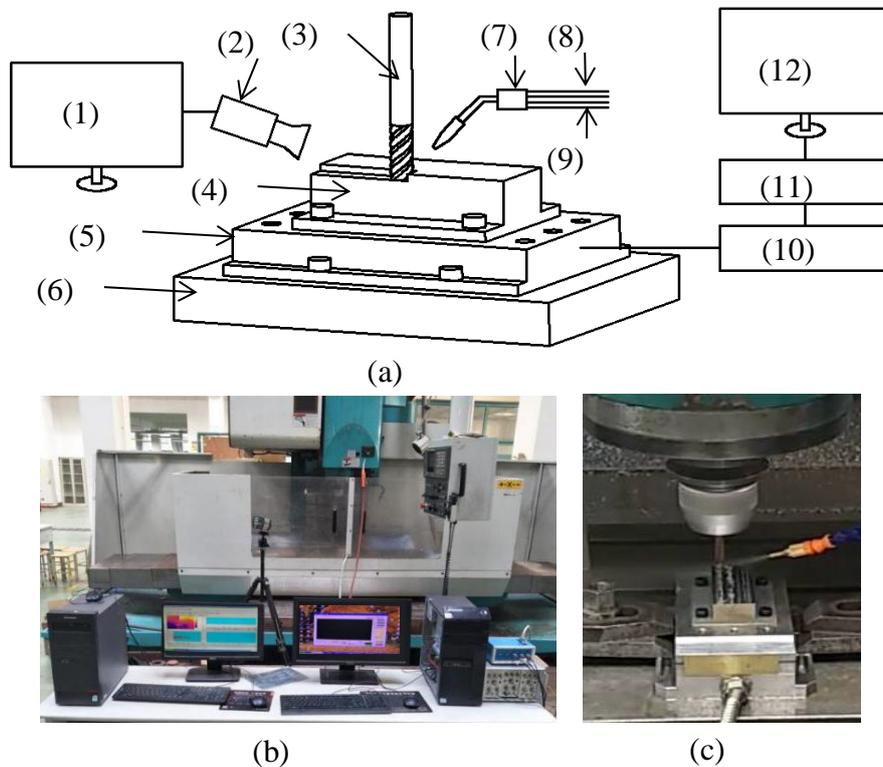
Fig. 1 Installation sketch of the milling test. b Installation physical drawing of the experimental measuring device. c Physical chart of the milling test process. (1) Milling temperature acquisition and analysis software; (2) infrared thermal imager; (3) milling cutter; (4) workpiece; (5) dynamometer; (6) machine tool workbench; (7) atomizer; (8) intake pipe; (9) cutting Fluid Pipe; (10) charge amplifier; (11) data acquisition instrument; (12) milling force acquisition and analysis software.
