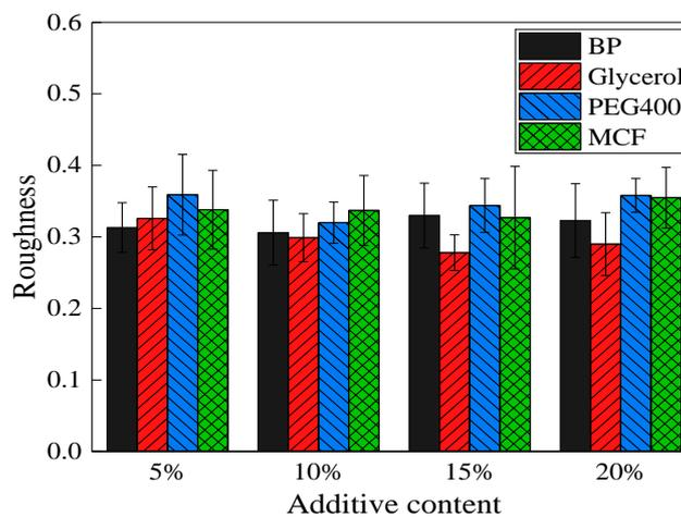
Fig. 6 Roughness synthetic figure of the four cutting fluids varying with content
