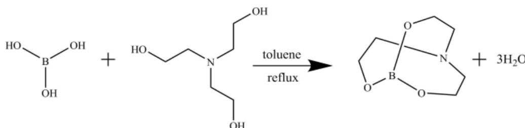
Fig. 13 Reaction formula of triethanolamine borate
