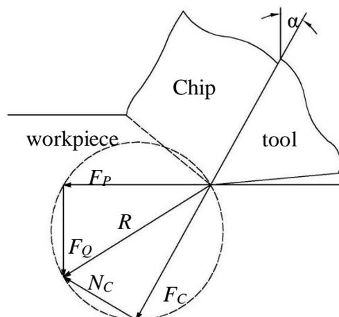
Fig. 8 Relation of forces in milling
