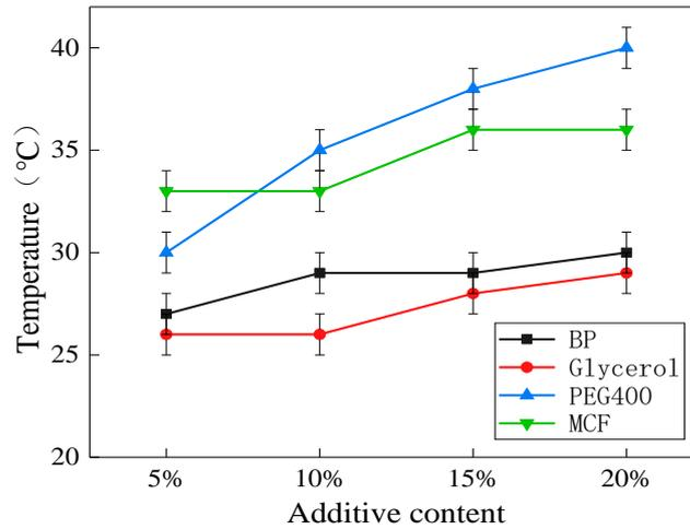
Fig. 3 Variation of the milling temperature of the four cutting fluids with the additive content
