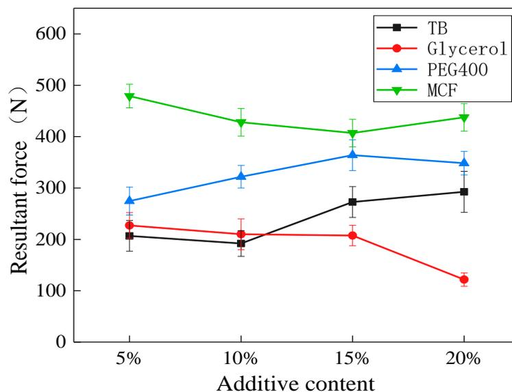
Fig. 2 Variation of the milling resultant force of the four cutting fluids with additive content
