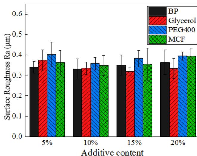
Fig. 4 Surface Roughness measured for the four kinds of cutting fluids at different contents
