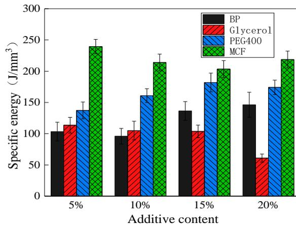
Fig. 7 Specific energy of the four cutting fluids with different additives
