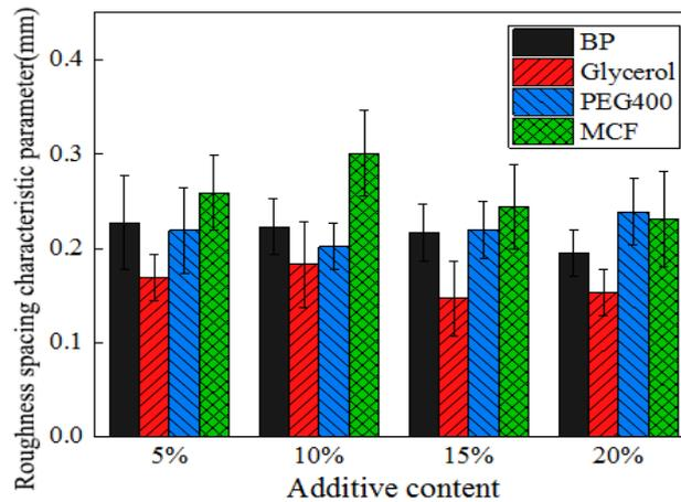
Fig. 5 RSm values of roughness measured for the four kinds of cutting fluids at different contents
