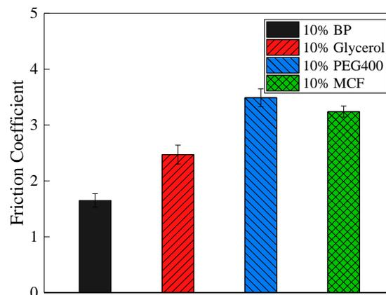
Fig. 9 Friction coefficients of the four cutting fluids at a 10% content
