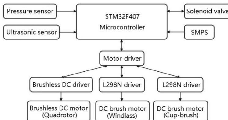
Figure 2. Structure diagram of control
