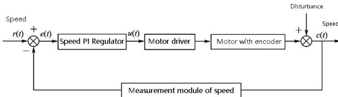
Figure 3. Block diagram of speed PI control system
