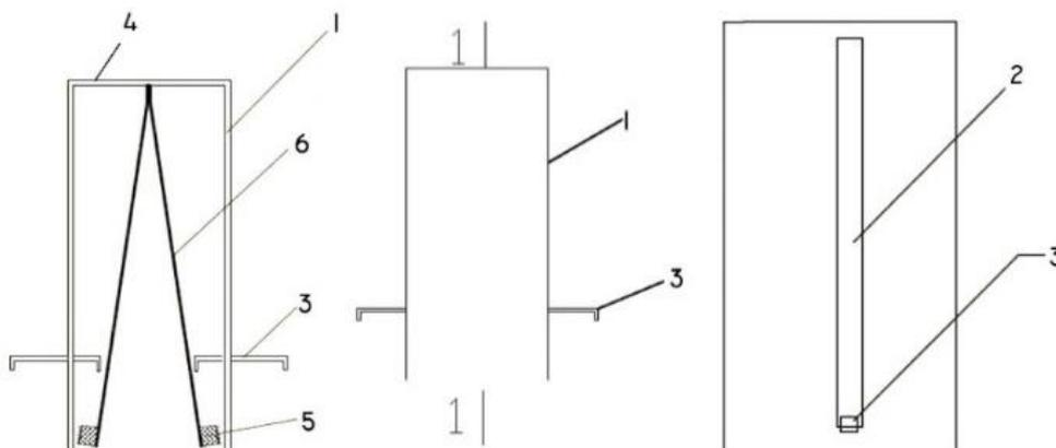
Figure 1. Preserved pipe end protection device for building electrical
