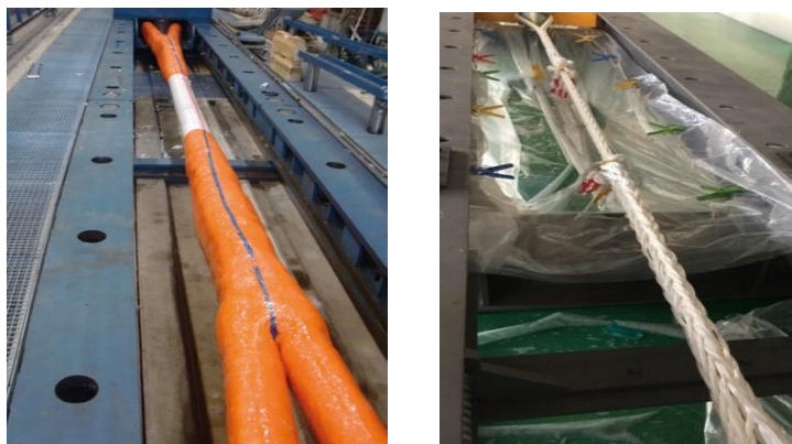
Fig. 3 Schematic diagram of polyester cable elongation (stiffness) test
