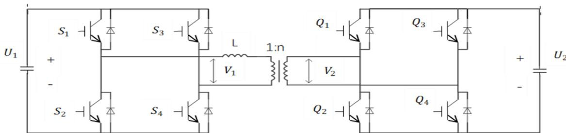
Fig. 10 DAB converter schematic
