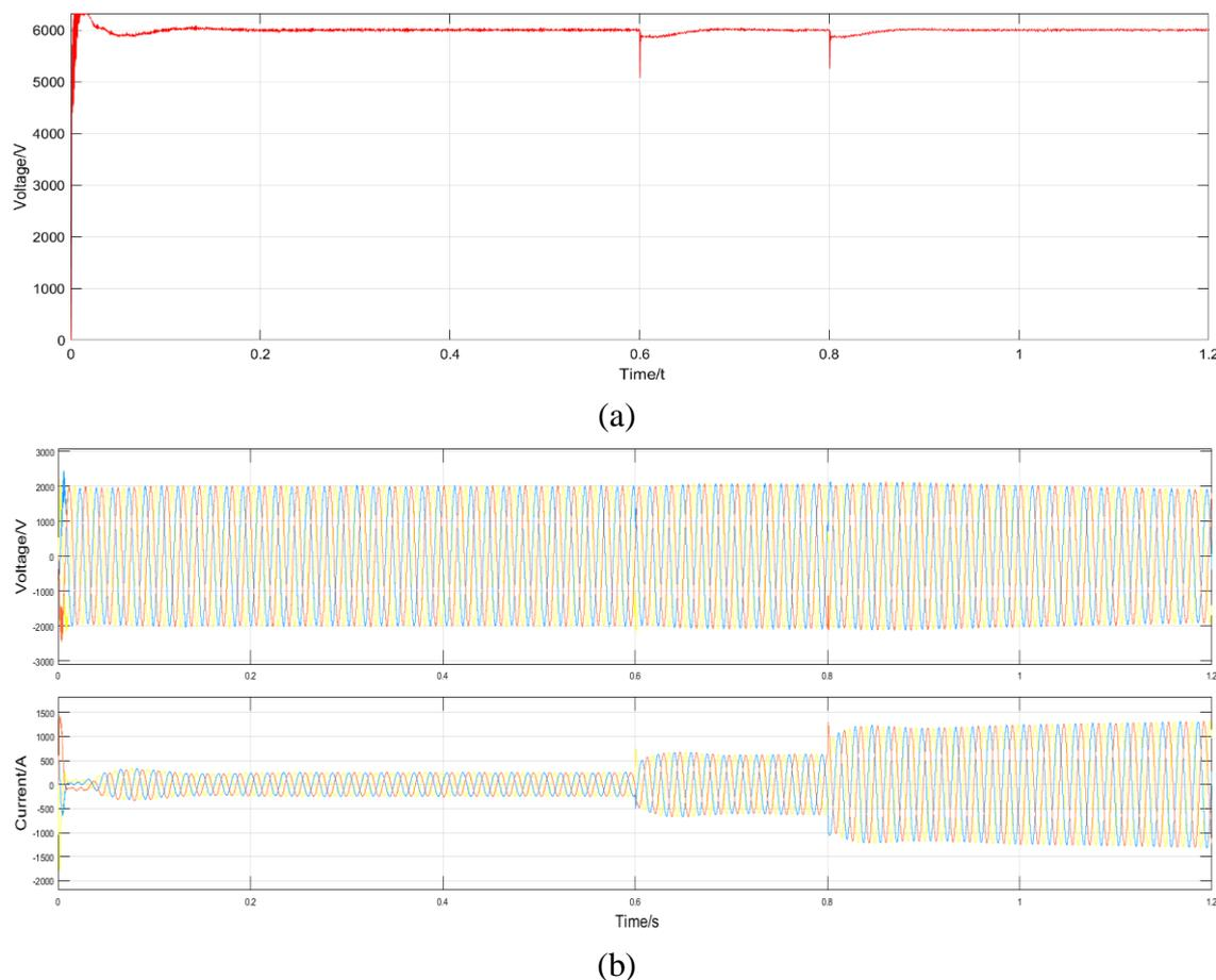
Fig. 13 (a)Bus voltage change, (b) The output voltage and current of the generator
