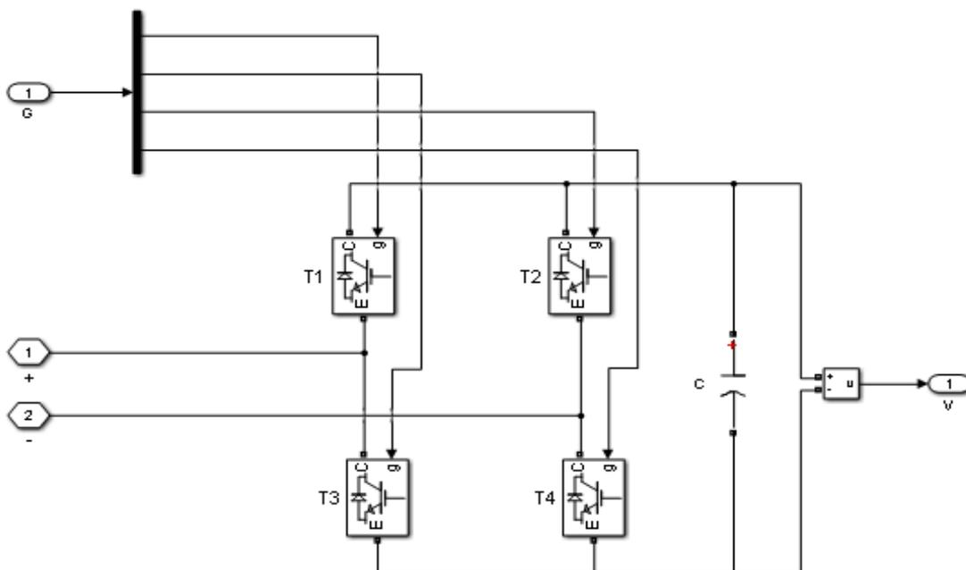
Fig. 7 Three-phase half-bridge converter topology
