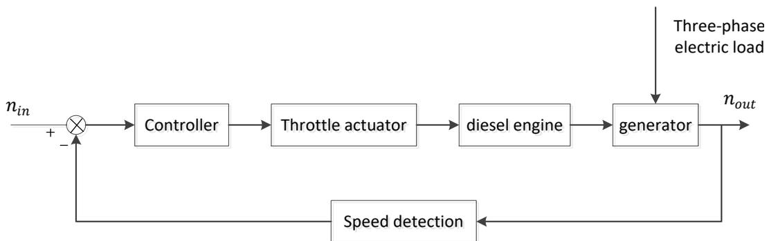
Fig. 2 Block diagram of the speed feedback control system of marine diesel generator set
