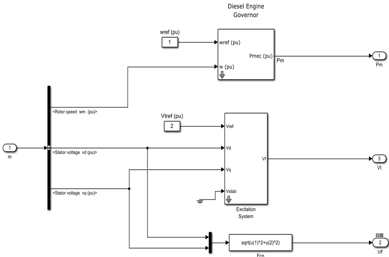
Fig. 5 Simulation model of diesel engine
