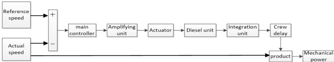
Fig. 3 Block diagram of diesel engine and governing system model
