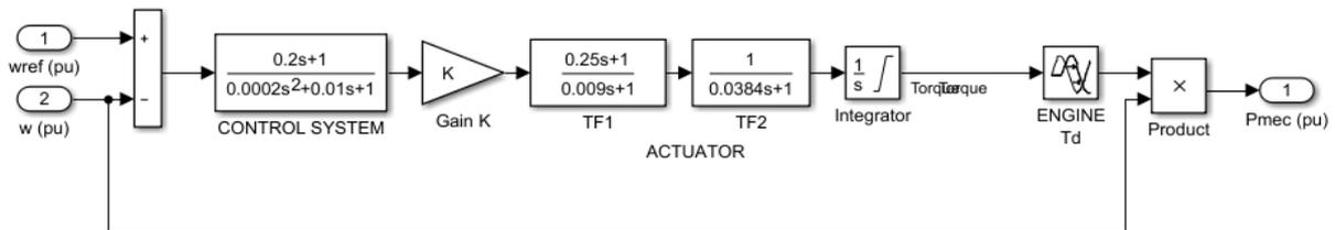
Fig. 4 Block diagram of speed control system
