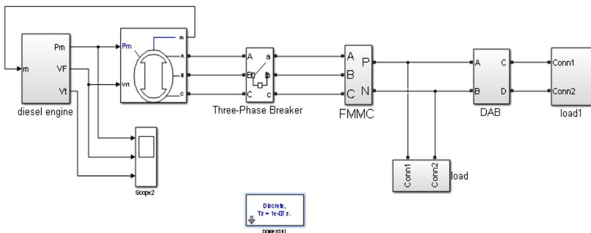
Fig. 11 Whole simulation model of ship power system
