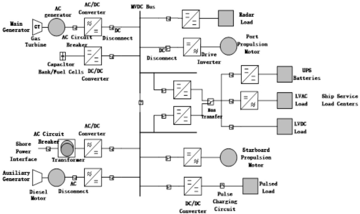
Fig. 1 Radial distributed framework
