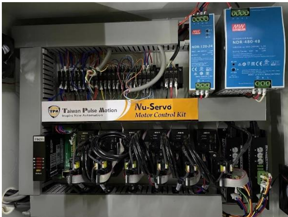
Fig. 4 Controller and drive integrated cabinet
