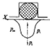
Fig. 2 Contact pressure distribution of sealing ring
