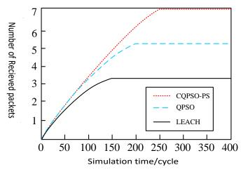
Fig. 10. Comparison of total packets transmitted by three protocols
