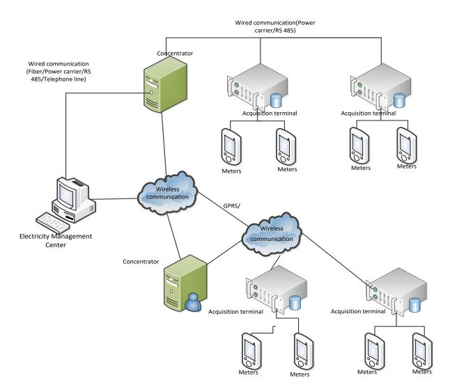
Fig. 1 Architecture of Data Communication Network Scheme for Urban Meters
