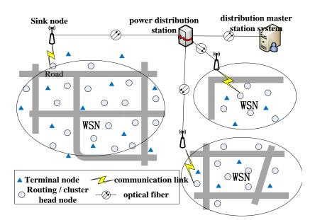
Fig. 3 Structure of wireless communication network platform for urban meter reading
