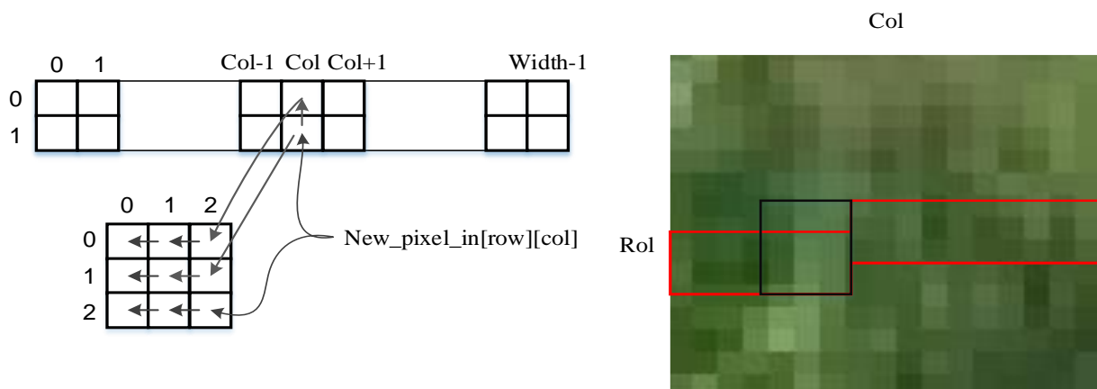
Fig. 1 Diagram of window buffer and line to achieve 2D convolution
