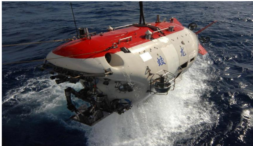
Figure 1. The 'Jiaolong' HOV with Multiple thrusters
