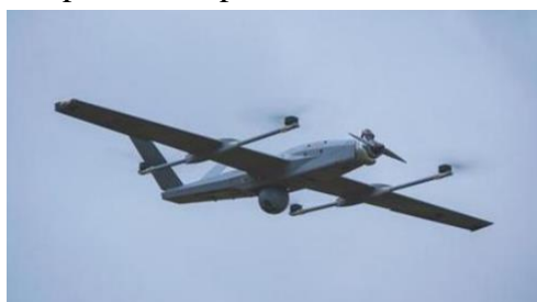
Fig2 A certain type of hybrid VTOL UAV
