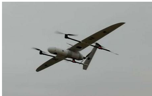
Fig4 Vertical take-off and landing test
