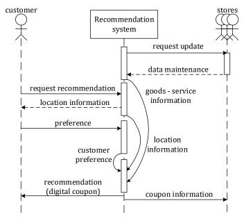
Figure 9. Sequence diagram of recommendation system
