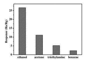
Fig. 4 Responses of the sensor to different VOC gases at 400°C
