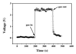
Fig.5 Response and recovery time of ZnSnO<sub>3</sub> sensor to 1000 ppm ethanol at 400°C
