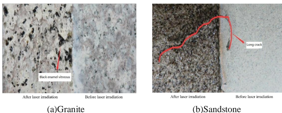
Figure 4 Contrast map of macroscopic appearance before and after action of linear spot
