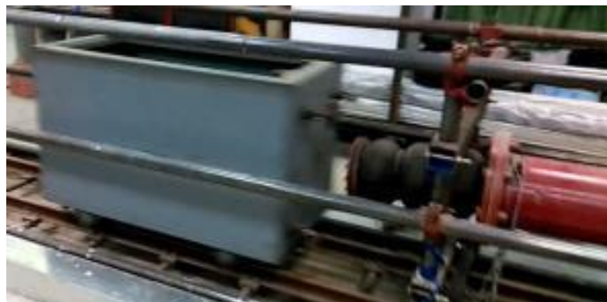
Fig. 8 ejection acceleration test bench of flexible cylinder
