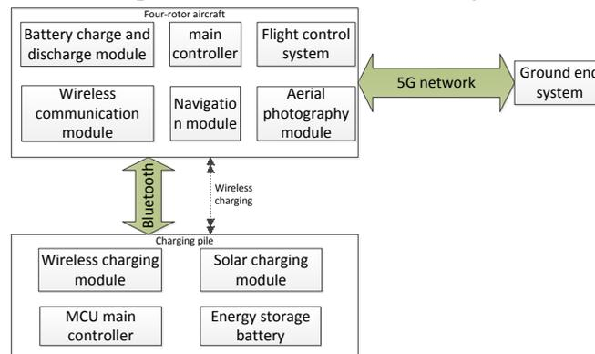
Fig. 1 System structure diagram
