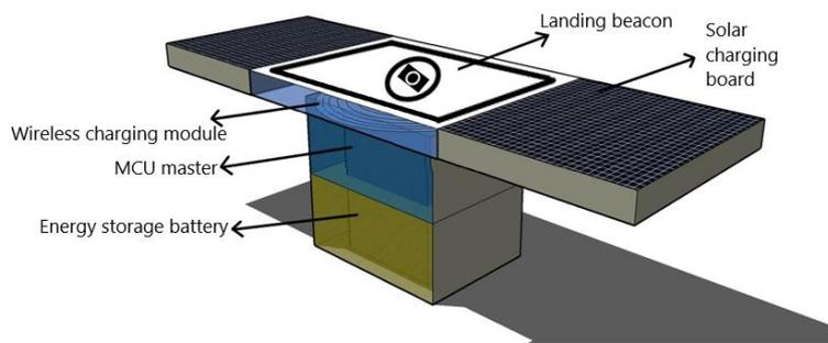
Fig. 6 charging pile model diagram
