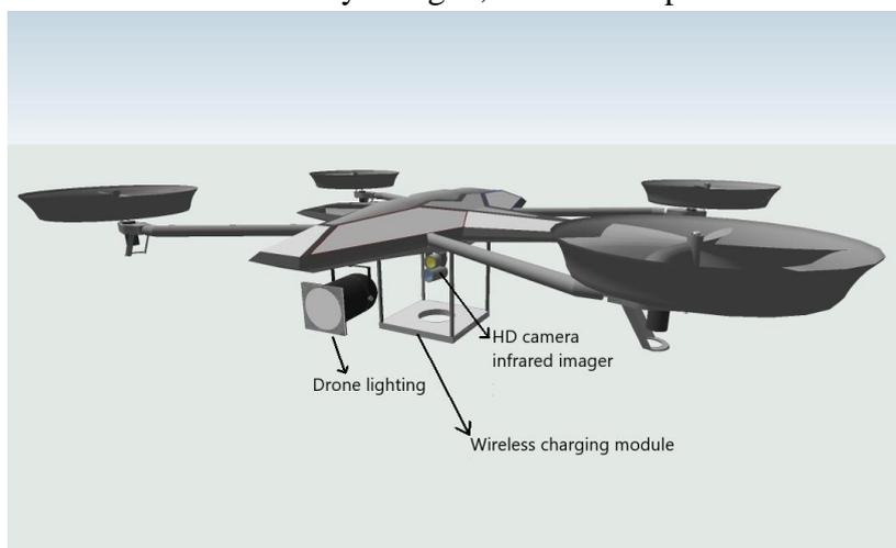
Fig. 4 drone model diagram
