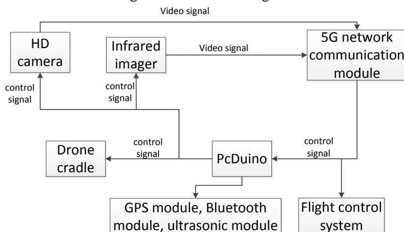
Fig. 5 UAV hardware structure diagram
