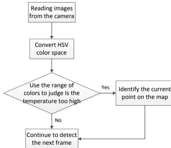
Fig. 13 infrared recognition process
