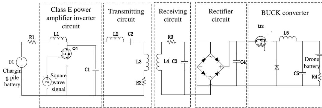
Fig. 11 Wireless charging circuit
