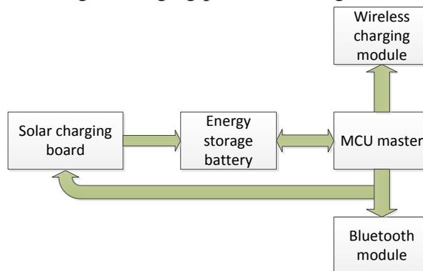
Fig. 7 charging pile hardware structure
