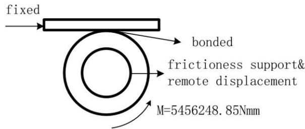
Figure. 2 Mechanics model of ZK worm and worm gear
