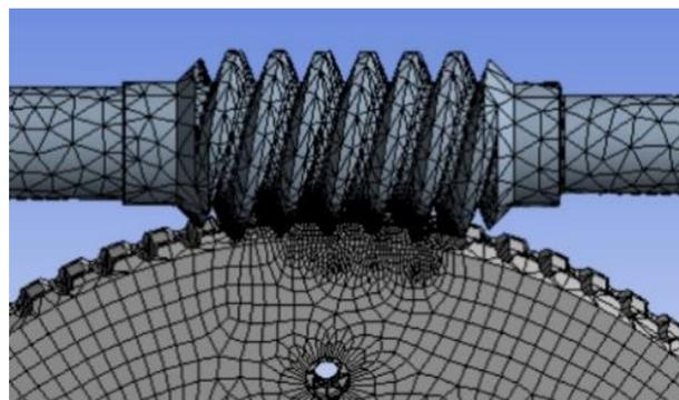
Figure. 3 ZK worm and worm gear wheel meshing mode
