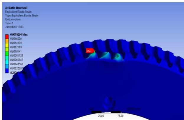
Figure. 5 ZK worm and worm gear equivalent strain cloud map
