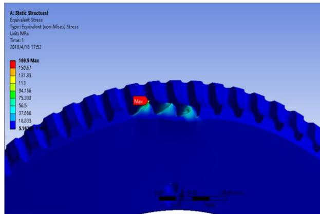
Figure. 4 ZK worm and worm gear equivalent stress map
