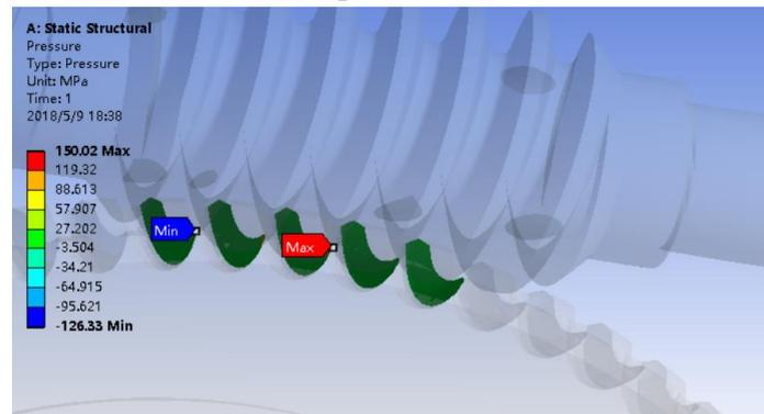
Figure. 6 Worm and worm gear contact position compressive stress cloud
