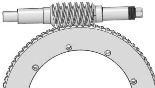
Figure. 1 Simplified model of ZK worm and worm gear
