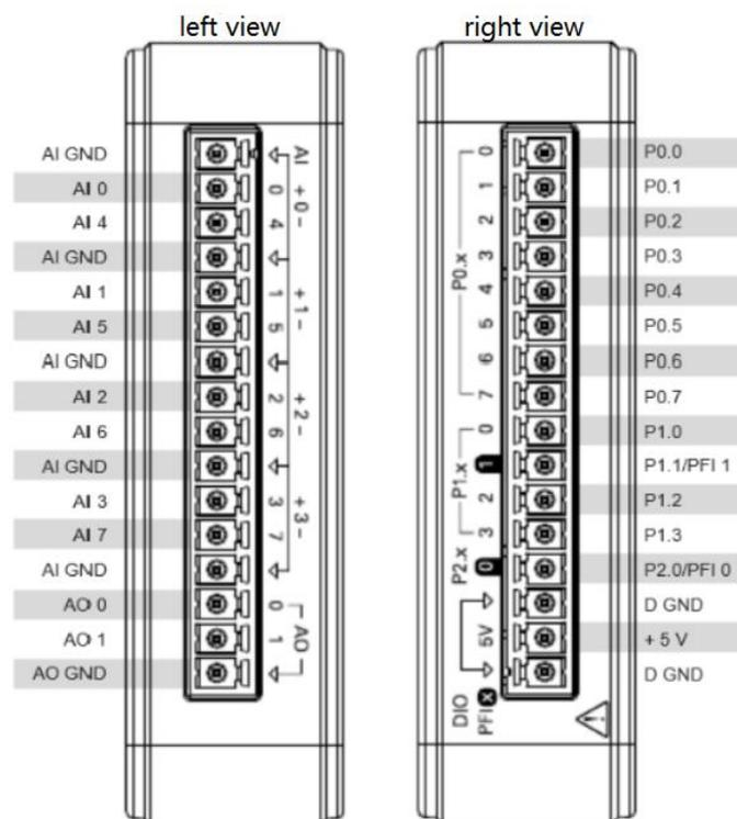
Fig.2 pin image of data acquisition card
