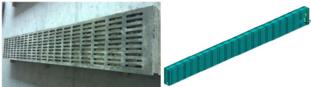
Fig. 2 A Concrete Noise Barrier Unit Plate B Simplified finite element model
