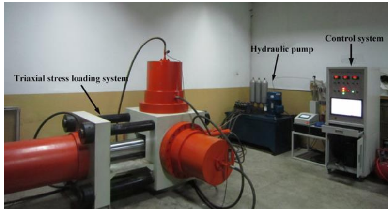
Fig.2 Hydraulic fracturing experimental device
