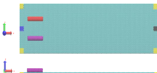
Fig. 3 Replacement of nanoparticles with double carbon nanotubes
