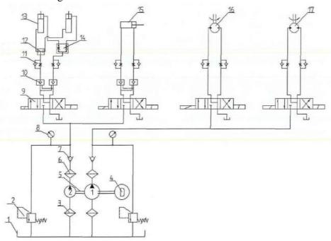
Oil tank 2.relief valve 3.purolator 4.Electric machinery 5.Bidentate united pump 6.purolator 7.Check valve 8.piezometer 9.Three - position four-way electromagnetic directional valve 10. Hydraulic lock 11 .flow speed control valve 12. joint 13. Movable arm oil cylinder 14.flow-combining valve 15. turn oil cylinder 16. Walking left motor 17.Walking right motor
