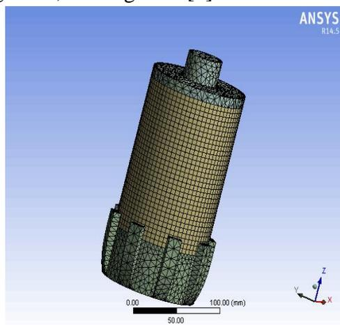
Fig. 5 Mesh division of fishing device
