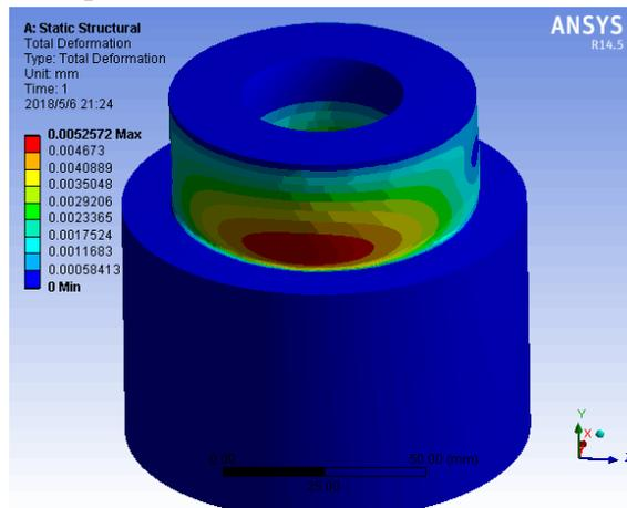
Fig. 11 Total deformation of the mother cone
