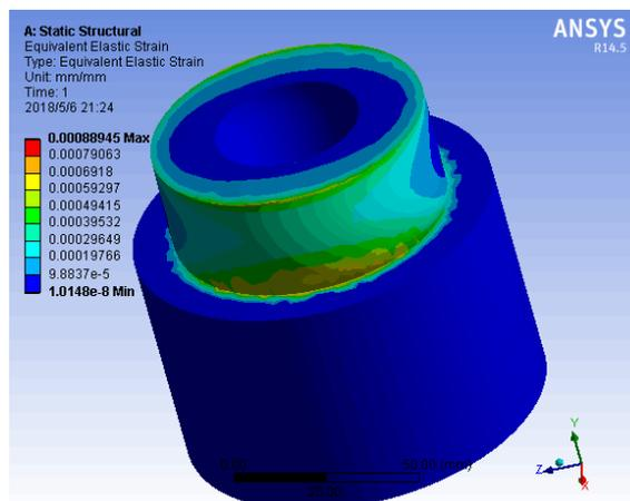
Fig. 12 Female cone strain cloud map
