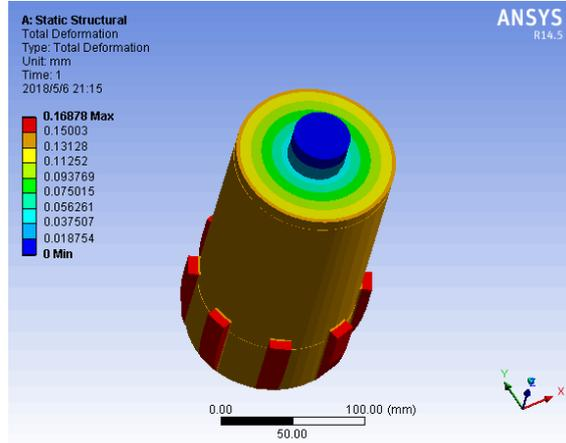
Fig. 8 Total deformation of the salvage device
