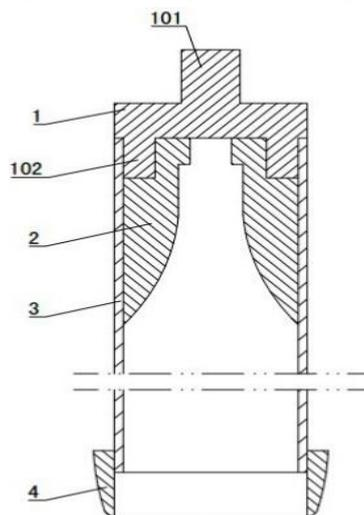
1—Coring tube seat; 101—Connecting part; 102—Installation section; 2—Female cones;
