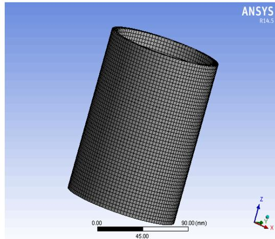
Fig.6 Meshing of core tube
