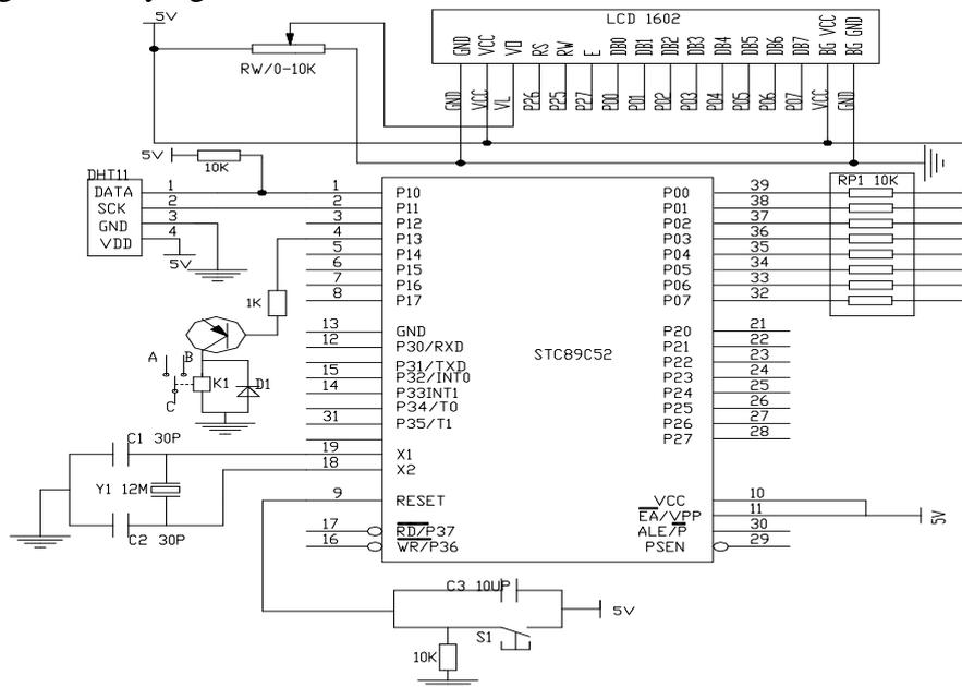
Figure3. Wiring Diagram for Control Circuit
