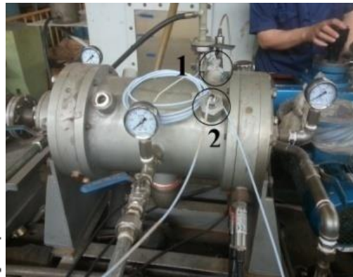
Figure 3. Schematic diagram of displacement sensor installation
