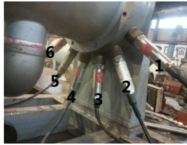
Figure 2. Schematic diagram of pressure sensor arrangement
