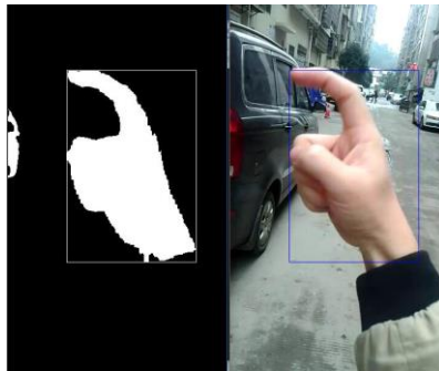
Figure 1. Elliptical skin model detection and extraction of gesture area
