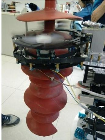
After cleaning the insulators of the layer, the robotic arm expands the maximum angle, the lifter lowers the corresponding insulator pitch, and the robotic arm buckles an insulator to open the cleaning. Repeat the fifth step until the bottom insulator is cleaned.
