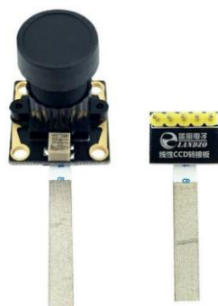
Fig 6. Linear Charge Coupled Device gray sensor
