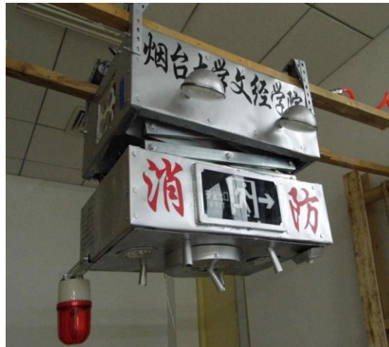
Fig 3. Security guard intelligent fire extinguisher
