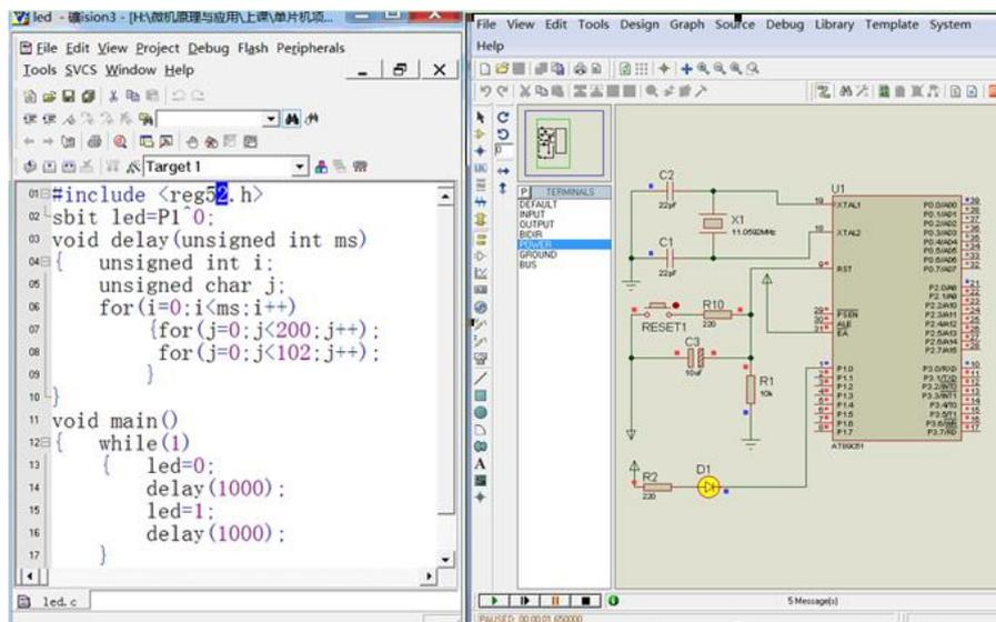
Fig. 2 Proteus Construction Virtual Hardware Circuit and Keil's C Language Programming
