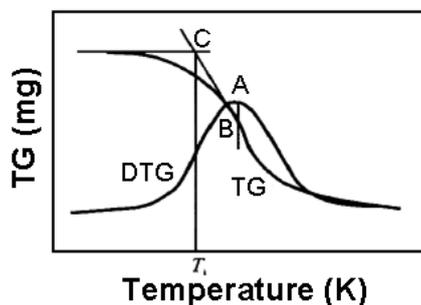
Fig.1. Schematic diagram of igniting temperature definition
