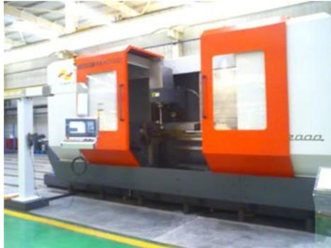
FIG.1 Spindle swing five-axis blade machining center
