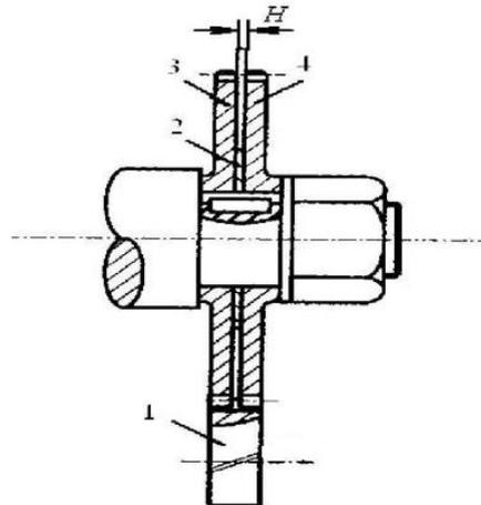
1, 3, 4: helical gear 2: Adjusting washer
