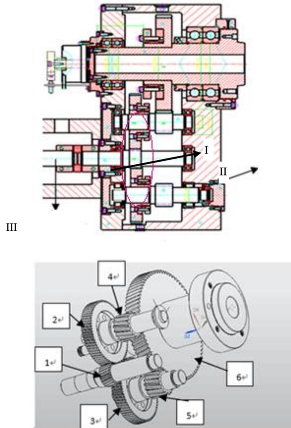
I-Double helical gear anti-backlash mechanism; II-Rehmannia automatic compensation mechanism;III-Input shaft
