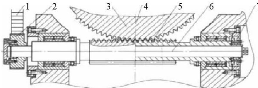
1-Toothed belt; 2-Toothed pulley; 3-turbine;4-Contact center; 5-Hollow worm; 6-Worm shaft; 7-Expansion sleeve
