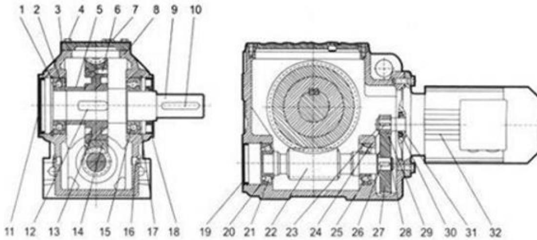
1.17.23.28-Retaining ring; 2.15.21.25.31-Bearing; 3.11.19-cover; 4-bolt; 5-Bushing; 6-Screw; 7-Vent cap; 8-Box; 9-Output shaft;10.12.24.26-Flat key; 13-Turbine mandrel; 14-Turbine rim; 16-Oil mirror;18.30-Oil seal; 22-Worm; 27.29-gear; 32-Motor
