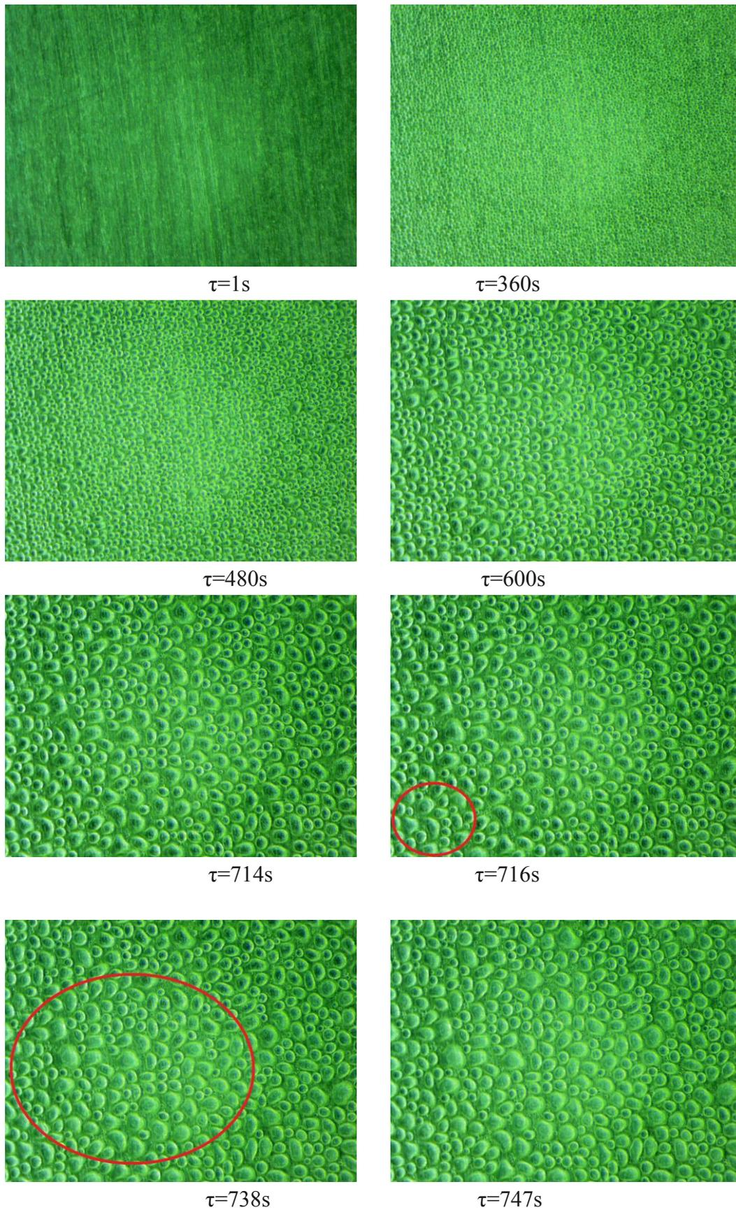
Fig. 3 Freezing process of water droplets  $T_{air}=13^{\circ}C$  RH50%
