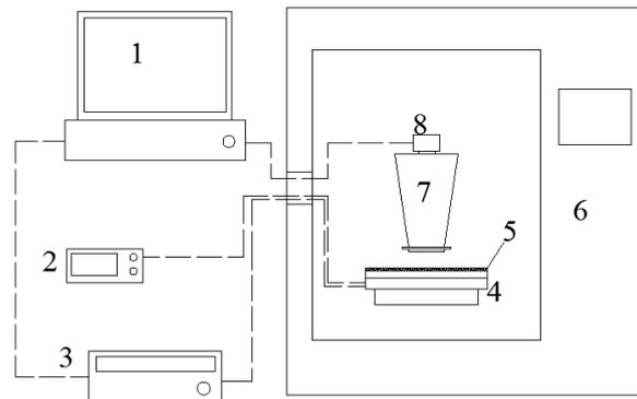
1:Computer; 2: Semiconductor refrigeration station thermostat; 3: Temperature collector; 4: Semiconductor refrigeration unit; 5: Aluminum sheet; 6: Constant temperature and humidity chamber; 7: Microscope; 8: CCD image collector
