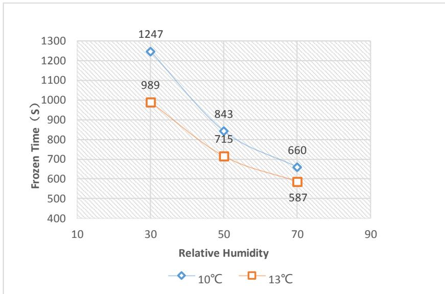
Fig. 4 Influence of environmental temperature and humidity on freezing time of water droplets
