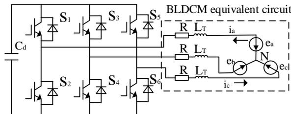
Fig. 4 Equivalent circuit of flywheel unit energy feedback braking
