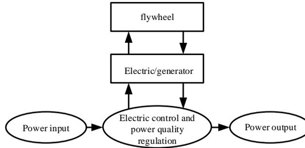
Fig. 1 Flywheel energy storage system working principle diagram
