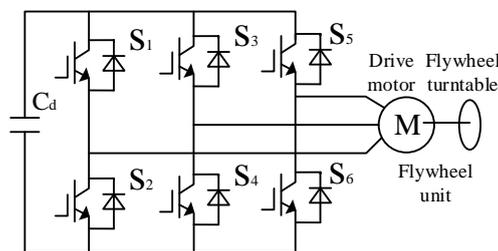
Fig. 3 Flywheel energy storage system power conversion main circuit topology
