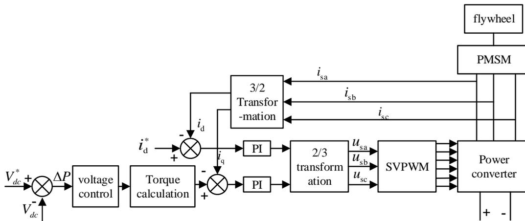
Fig. 2 Schematic diagram of discharge operation control principle
