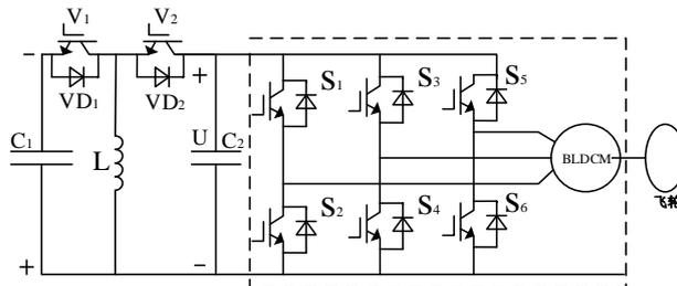
Fig. 6 Conversion circuit of permanent magnet brushless DC motor with bidirectional buck-boost Reference [21] proposes a simplified DC-DC conversion circuit that uses a bidirectional buck-boost design to remove V1 of Figure 6, leaving only the freewheeling diode VD1. When the motor is running
