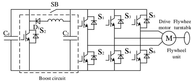
Fig. 5 Main circuit topology of flywheel energy storage system with boost circuit
